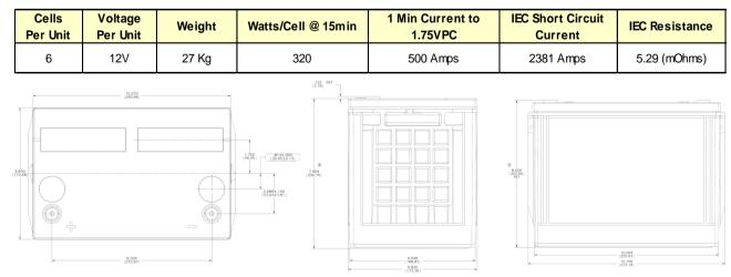
\*All dimensions in inches and (millimeters). All dimensions are for reference only. Contact a C&D Representative for complete dimensional information.
